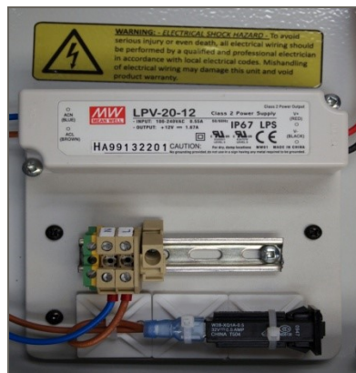
Figure 16: AC power supply terminal block
