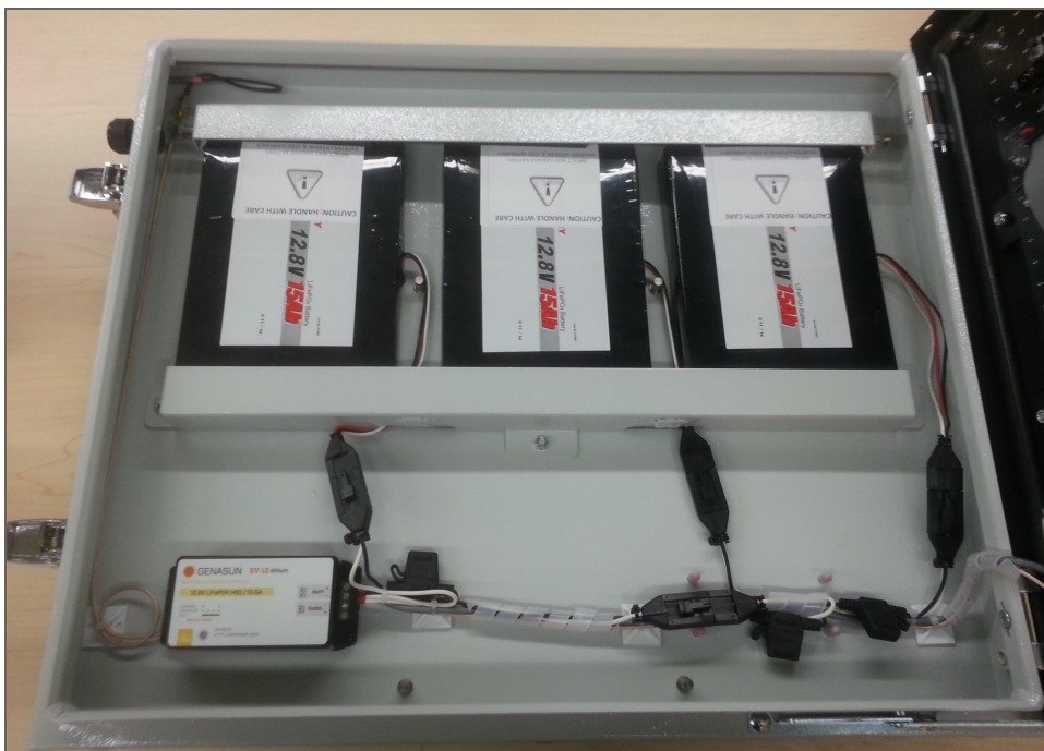
Figure 18: Batteries inserted and connected
